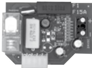
The time for the complete recharge of 12Vdc 1,2Ah batteries (n° 2 pieces connected in series, optional cod. ACG9511), at the first installation is of 24 hours, with a charge current of 0,03A.
